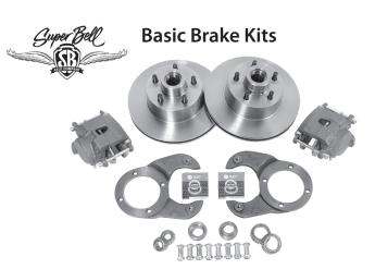
Super Bell's Basic Brake Kit adapts most '78-'86 intermediate passenger car GM calipers and rotors to '37-'48 Ford passenger car spindles.
