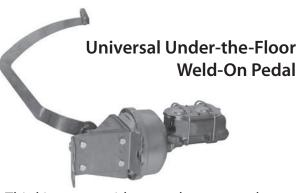
This kit comes with a new booster and master, pedal assembly, and necessary hardware. BTSPK502 \$325.00
