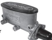
High-pressure die casting of a premium alloy produces a high-capacity body with a black anodized, machined billet lid that captures a pressure balanced bellows gasket with 100% sealing against moisture invasion or fluid leakage. The mounting flange is slotted to accommodate installation on bolt centers between 3.22" and 3.40". Please specify 1" or 1 1/8" bore.
